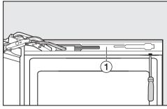
Remove panel ① from the soft-close mechanism by inserting a flat-bladed screwdriver into the gap from above and easing it off bit by bit.
